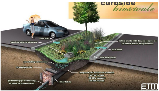
Bioswale absorbs runoff and channels excess toward the storm drain in the lower lot.
